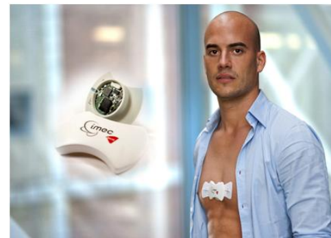
Bluetooth wireless electrocardiogram patch and posture monitoring device with imec's ultra low power SOC; photo: imec
