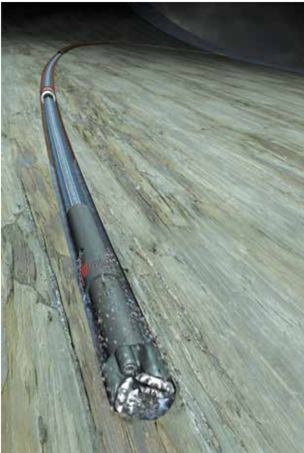
FIG 9: DUAL-WALL DRILLSTRING ULTRA-ERD CONCEPT
