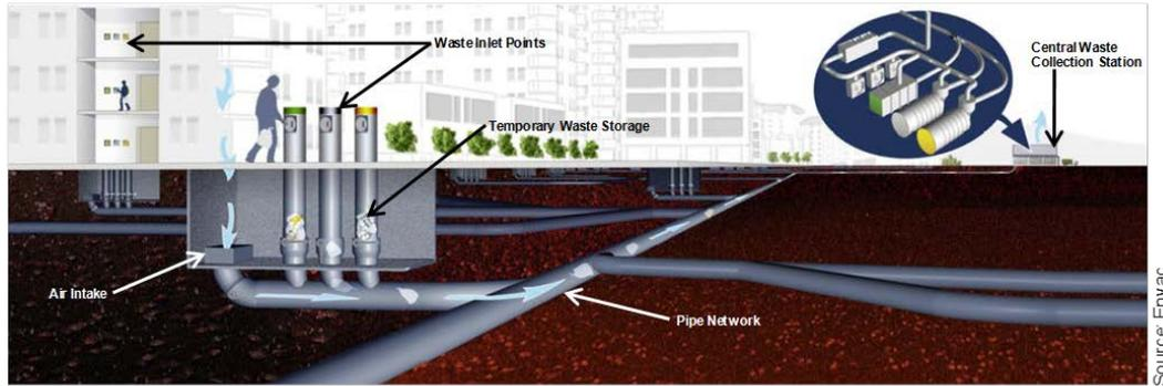
Figure 4.5: An illustration of an Automated Waste Collection Systems system
